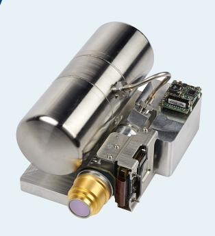
CRYASSY Focus is a miniaturized IDCA (Integrated Dewar Cooler Assembly) cryogenic assembly. Comprising a miniaturized pulse tube, detector and cryostat, it is designed for nanosat and microsat platforms.
