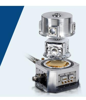
ACE-CUBE is a cryogenic platform operating in a closed cycle. Versatile, it is designed for low-temperature scientific instrumentation.
