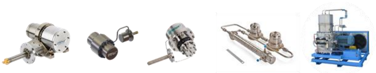
Figure 1. Example of different cryocoolers developed and produced by Absolut System (from left to right: LPT6510 2 W @ 80 K Pulse tube with TCBV, 0.5 W @ 130 K High frequency Pulse Tube, 0.5 W @ 150 K Joule-Thomson, 2 W @ 40 K turbo-Brayton, 1500 W @ 77 K High capacity Pulse tube)
