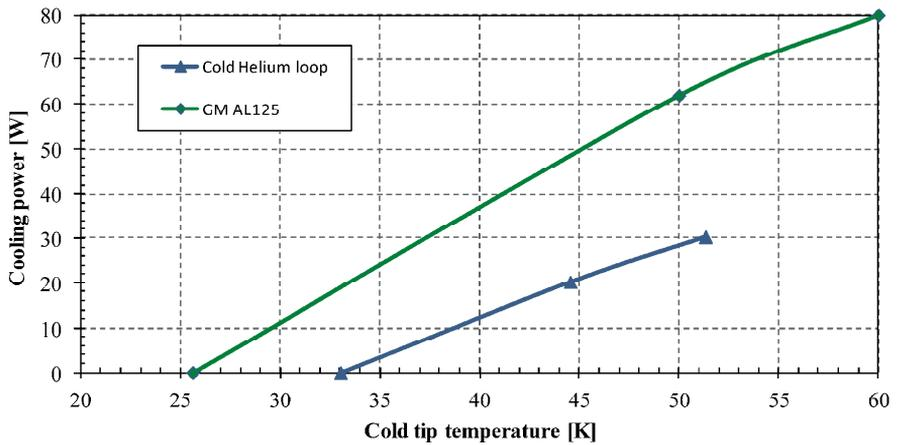
**Figure 6.** 50 K remote cold helium cooling loop performance test results and confrontation to the stand alone GM AL125 cold head.
