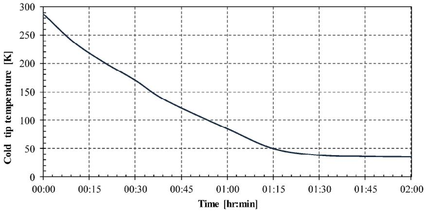
**Figure 5.** 50 K remote cold helium cooling loop test - cool down curve.
