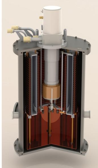
**Figure 9.** CAD cut view of the 30 K cold helium cooling loop cryostat.
