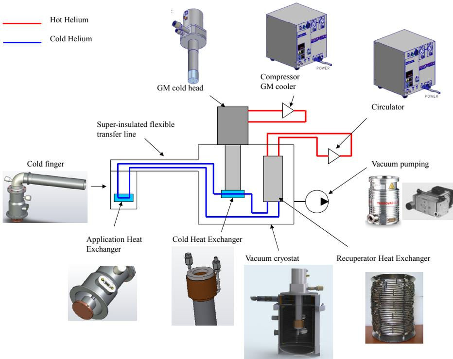
**Figure 1.** Schematic representation of the 50 K remote Helium cooling loop.
