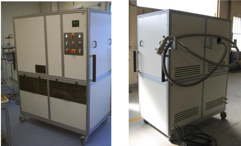
**Figure 4.** Final delivered 50K remote helium cooling loop installed into a mobile rack.
