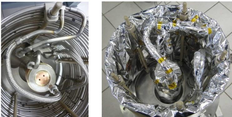
**Figure 2.** Tube-in-tube recuperator heat exchanger wound around the AL125 cold head and connected to the cold heat exchanger (with and without MLI insulation).
