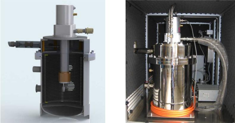
**Figure 3.** CAD cut view of the vacuum cryostat with the GM AL125 cold head and recuperator heat exchanger (left) and vacuum cryostat integrated in the cabinet (right).
