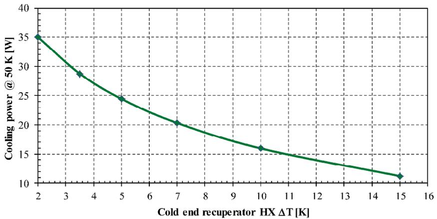
**Figure 7.** Cooling power at 50 K versus recuperator heat exchanger performance.
