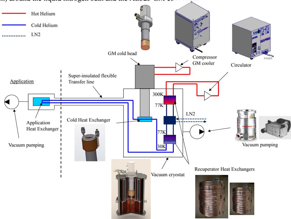
**Figure 8.** Schematic representation of the 30 K remote helium cooling loop.
