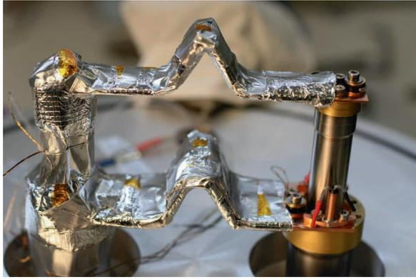
**Figure 8.** Cold redundant parasitic heat losses test bench. Left: coax DM cooler ON , Right: CNES EM cooler OFF.
