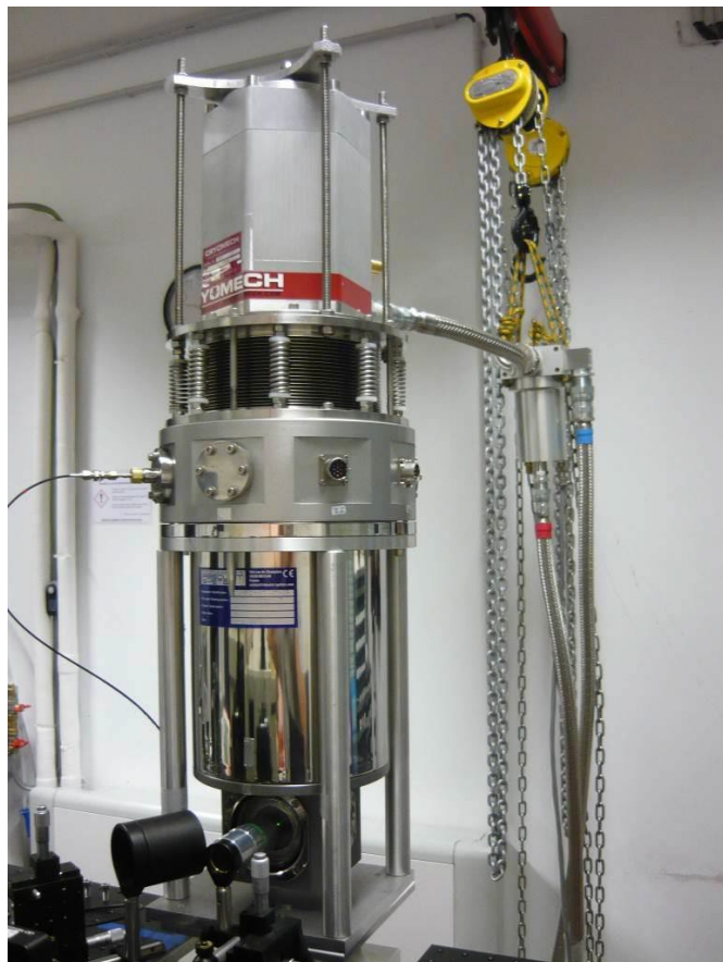
FIGURE 7. 2 stages pulse tube optical cryostat for Raman e electronic spectroscopy. (Laboratoire Matériaux et Phénomènes Quantiques, University Paris Diderot – Paris VII)
