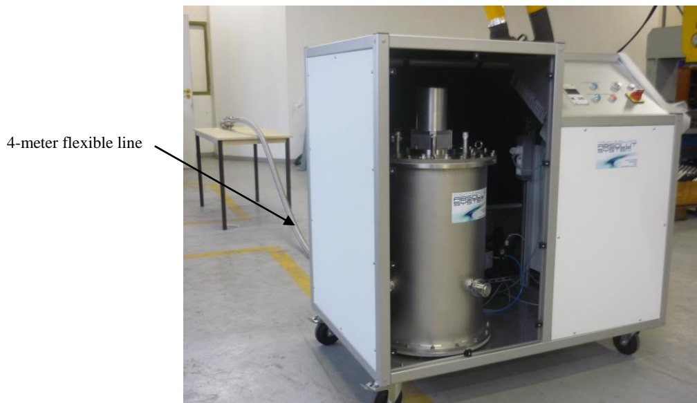
FIGURE 9. Helium cooling loop cryostat integrated inside a cabinet.
