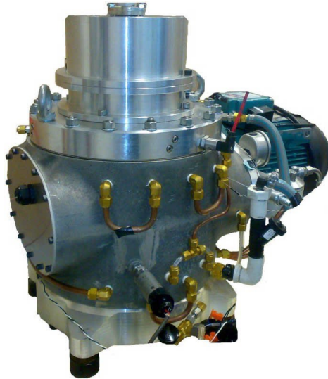
Figure 2. The CHC90 PWG with PT100 Beta pulse tube inside cryostat.
