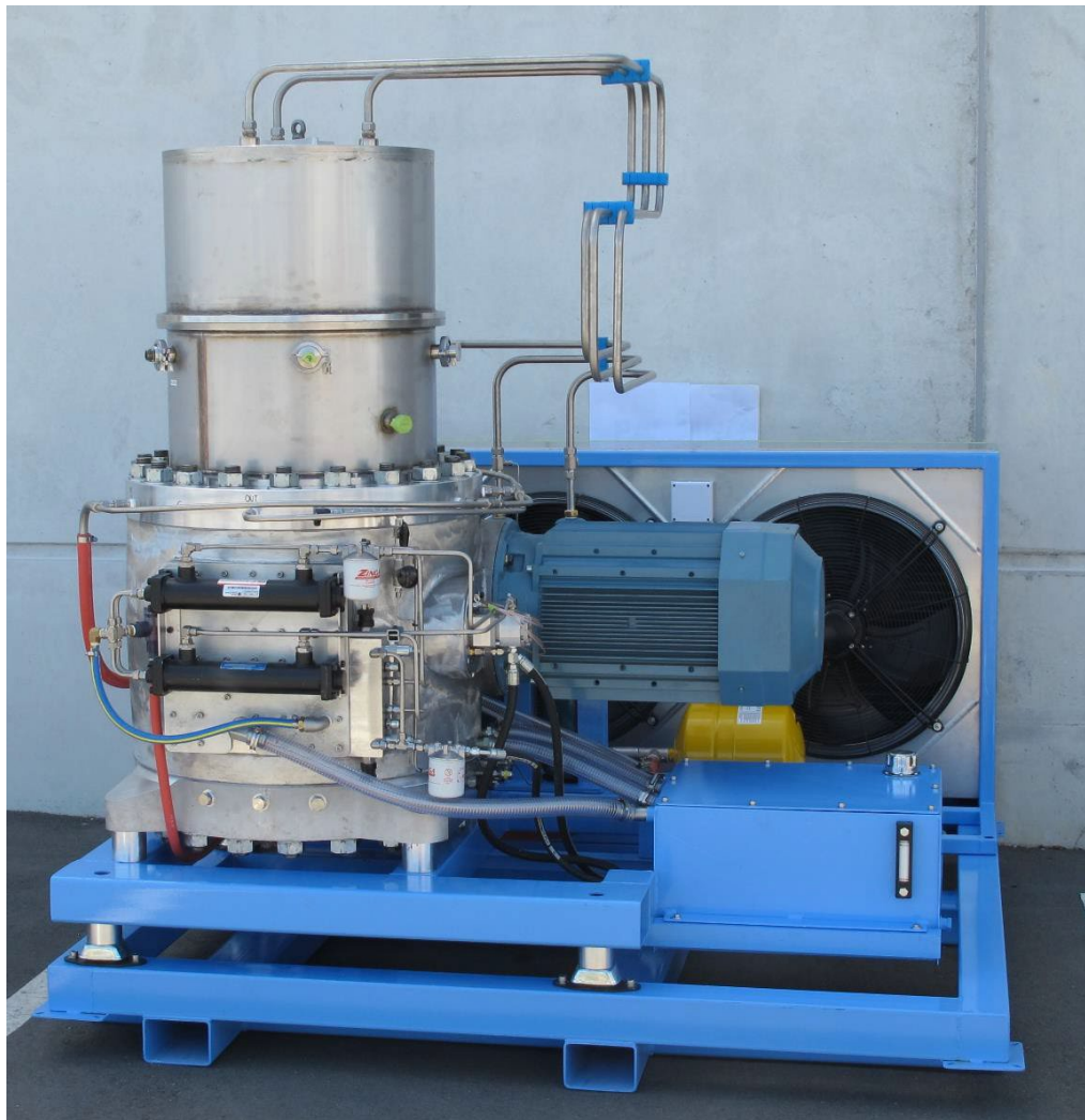
Figure 1: The PTC1000 beta cryocooler, including air cooling and mounted on a subframe ready for integration into a liquefier.
