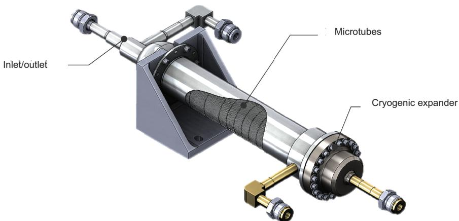
**Figure 6.** Recuperator design with integrated cryogenic expander
