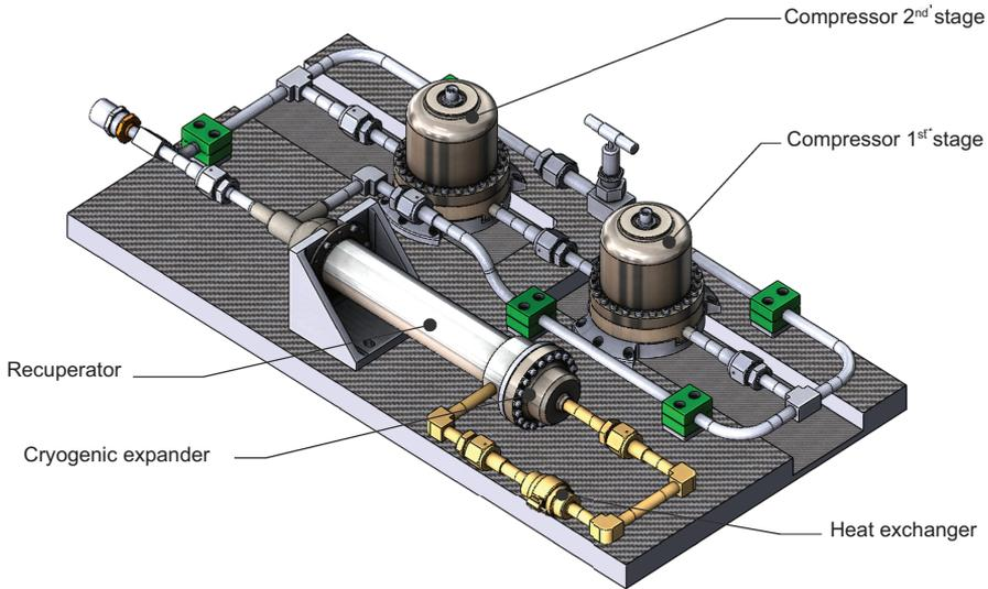
**Figure 2.** Overview of the 40-80 K vibration free cooler
