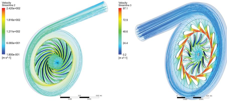
**Figure 4.** CFD Model (using CFX) showing streamlines (compressor on the left, expander on the right)
