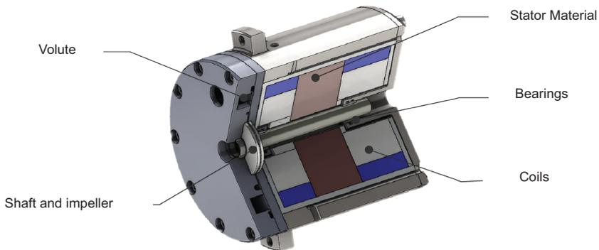
**Figure 3.** View of the compressor cartridge
