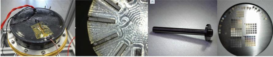
**Figure 8.** Breadboard samples: stator sample, dummy impeller, dummy shaft for hard coating, grooves manufacturing optimization
