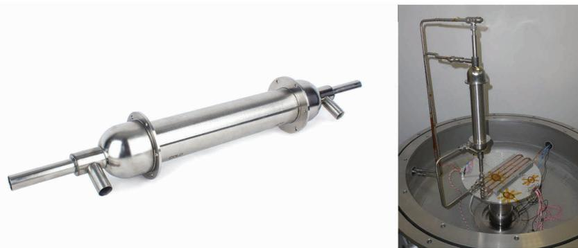
Figure 7. Picture of the recuperator prototype and test set-up in vacuum test chamber
