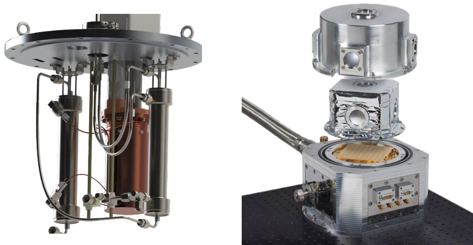
Figure 7. View of the interior of the cold box prior to MLI wrapping (left) and two stage table –top cryostat coupled to the 10 K remote helium cooling loop (right).
