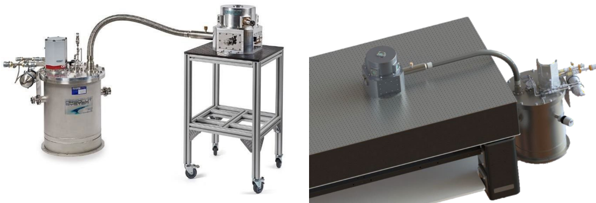
Figure 6. Left: 10 K two stage remote Helium cooling loop and cryostat produced. Right: Illustration example of the cryostat configuration on the optical table.
