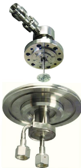
Figure 3. Picture of the Cryozone Noordenwind type cryofan used as the circulator.
